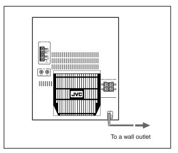
When connecting the AC power cord into a wall outlet, the unit automatically starts display demonstration.
