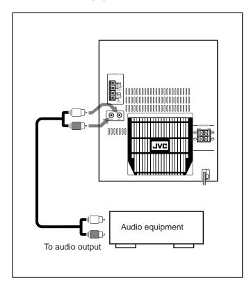
Connect the audio output jacks on the other equipment and the AUX jacks on the rear, using an audio cord (not supplied).
